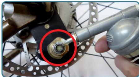
Slightly pull one of the shifter cables while mounting the shiftbox to align the hexagonal shiftbox interface and the hubs hexagonal shaft.
