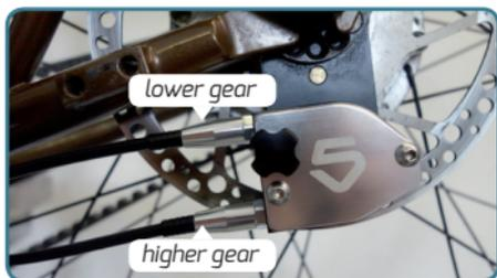
Therefore you can choose your desired shifting logics by connecting the shifter cable to either the right or the left gear lever on your handle bar.
