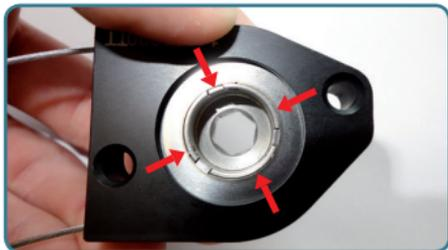
10. Rotate the housing cover around the locking screw until the outer demeshing plate is fully visible. Position the outer demeshing plate on the housing and center the borehole onto the shifting unit.
