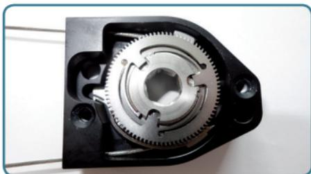
9. The shifting unit has to be centered into borehole of the inner demeshing plate. Pay attention to not bending any parts such as the catch by improper handling.
