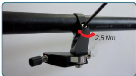
2. Mount the shiftbox onto the hub's hexagonal interface bolt. The hub's gear position has no significance. Apply a small amount of grease onto the hub's shifting shaft to ensure easy sliding between shaft and the shiftbox interface during installation.
