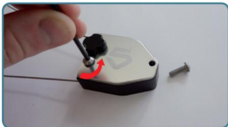
4. Remove the switching unit from the housing. It consists of the shifting hex cylinder, 2 tooth rings, 2 ratchets and 2 cable seats.
